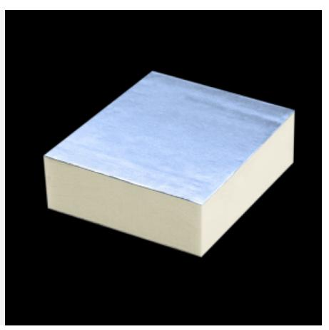
**POLIISO® AIR CARE GA080** is a sandwich panel consisting of a yellow-colored, closed-cell rigid polyiso (polyurethane foam) foam expanded between two aluminum supports: that of the outer face in 80-µm embossed aluminum and that of the inner face in 80-µm antibacterial smooth aluminum.
