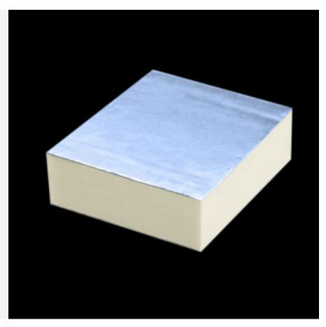
**POLIISO® AIR CARE GA200** is a sandwich panel consisting of a yellow-colored, closed-cell rigid polyiso (polyurethane foam) foam expanded between two aluminum supports: that of the outer face in 80-µm embossed aluminum and that of the inner face in 200-µm antibacterial smooth aluminum.
