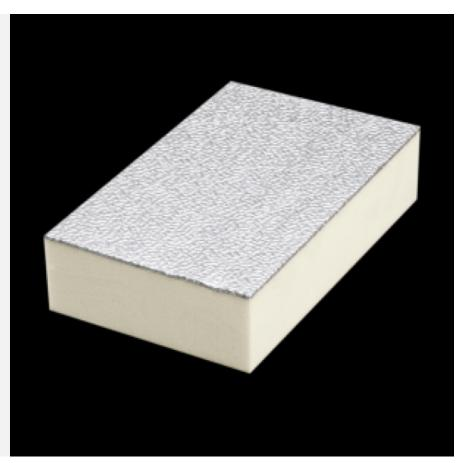
**POLIISO**® **AIR INDOOR GG080** is a sandwich panel consisting of yellow, closed-cell rigid polyiso (polyurethane foam) foam expanded between two 80-µm embossed aluminum supports.
