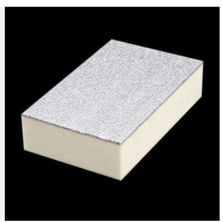
**POLIISO**® **AIR INDOOR GG200** is a sandwich panel consisting of yellow-colored, closed-cell rigid polyiso (polyurethane foam) foam expanded between two embossed aluminum supports: that of the outer face 200  $\mu$ m and that of the inner face 80  $\mu$ m.
