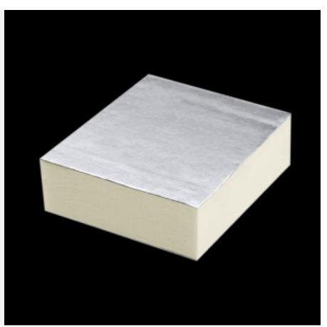
**POLIISO® AIR INDOOR GL200** is a sandwich panel consisting of yellow-colored, closed-cell rigid polyiso (polyurethane foam) foam expanded between two aluminum supports: that of the outer face in 80-µm embossed aluminum and that of the inner face in 200-µm smooth aluminum.
