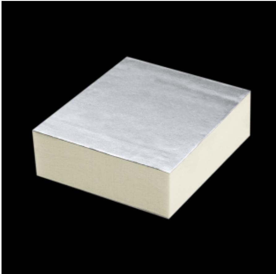
**POLIISO® AIR INDOOR GL400** is a sandwich panel consisting of yellow-colored, closed-cell rigid polyiso (polyurethane foam) expanded between two aluminum supports: that of the outer face in 200-µm embossed aluminum and that of the inner face in 200-µm smooth aluminum.
