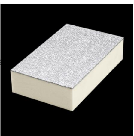
Panel coated on both sides with an 80-µm embossed aluminum foil to which a special lacquer coating is applied, giving the product exceptional resistance to highly corrosive substances such as chlorine and salt. This feature makes the product versatile to installation in particularly aggressive environments such as swimming pools, spas, maritime premises and other saline environments.
