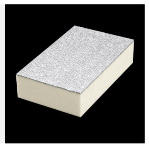
**POLIISO**® **AIR OUTDOOR GG080** is a sandwich panel consisting of yellow, closed-cell rigid polyiso (polyurethane foam) foam expanded between two 80-µm embossed aluminum supports.
