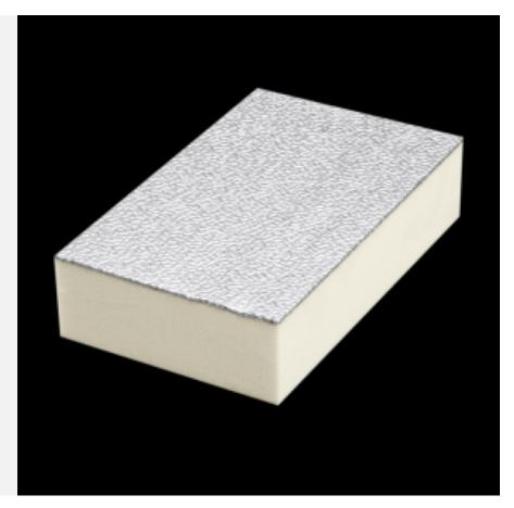
**POLIISO® AIR OUTDOOR GG200** is a sandwich panel consisting of yellow-colored, closed-cell rigid polyiso (polyurethane foam) foam expanded between two embossed aluminum supports: that of the outer face 200  $\mu$ m and that of the inner face 80  $\mu$ m.
