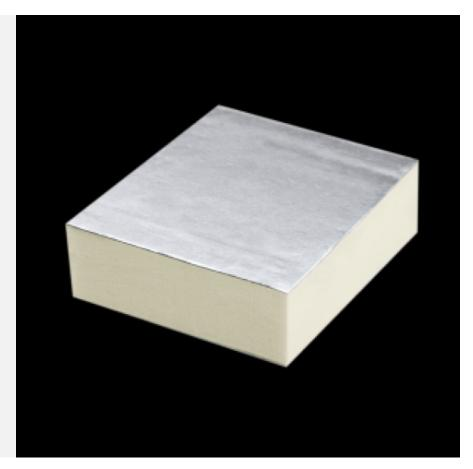
**POLIISO® AIR OUTDOOR GL080** is a sandwich panel consisting of yellow-colored, closed-cell rigid polyiso (polyurethane foam) foam expanded between two supports: that of the outer face made of 80-µm embossed aluminum and that of the inner face made of 80-µm smooth aluminum.
