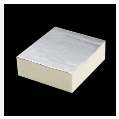
**POLIISO® AIR OUTDOOR GL200** is a sandwich panel consisting of yellow-colored, closed-cell, rigid polyiso (polyurethane foam) foam expanded between two aluminum supports: that of the outer face in 80-µm embossed aluminum and that of the inner face in 200-µm smooth aluminum.
