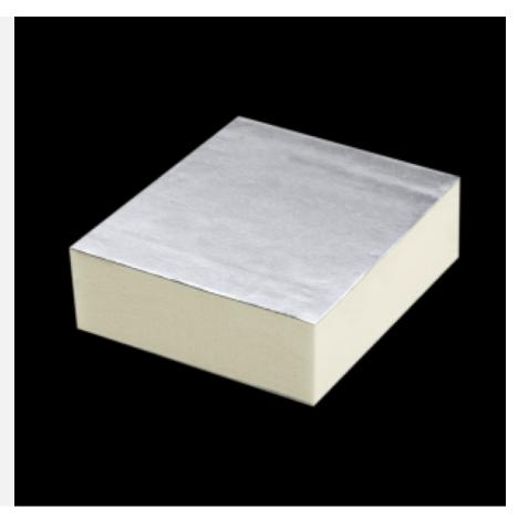
**POLIISO® AIR OUTDOOR GL400** is a sandwich panel consisting of a yellow, closed-cell, rigid polyiso (polyurethane foam) expanded between two aluminium supports: the outer face in 200  $\mu$ m embossed aluminium and the inner face in 200  $\mu$ m smooth aluminium.
