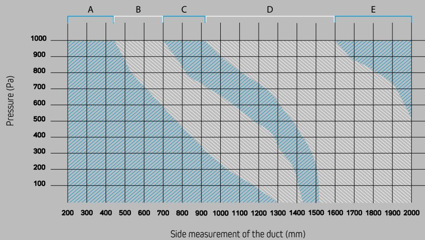
A: reinforcement bars not necessary
