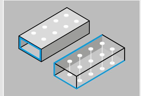
Figure 15: Application of 2 reinforcement bars
