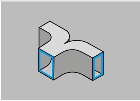
Figure 13: Two way elbow derivation
