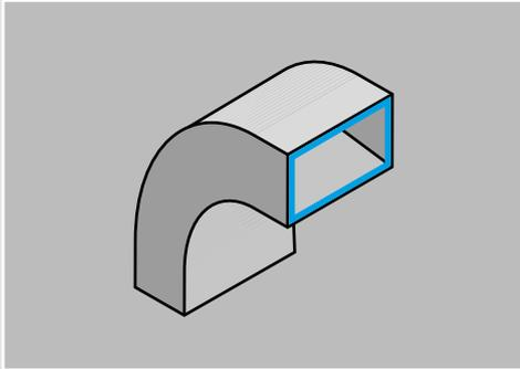
Figure 3 : Elbow with radius
