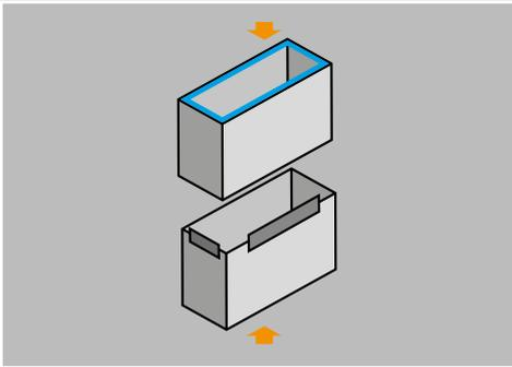
Figure 23: PVC bayonet mounting
