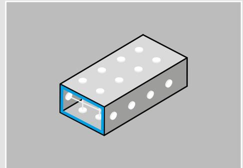
Figure 16: Application of reinforcement bars on all sides
