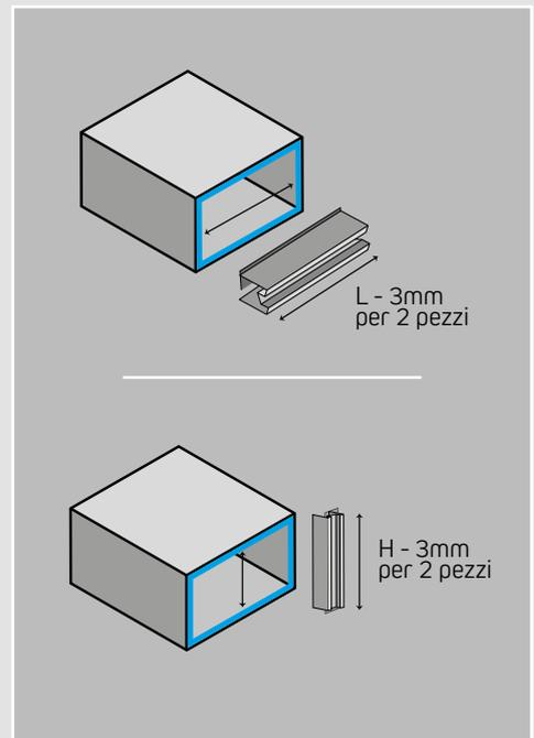
Figure 22: Invisible flange mounting
